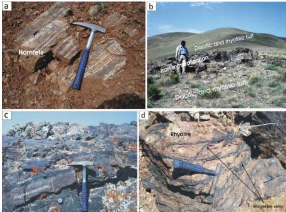
Fig.8: a) Dacitic and rhyolitic tuffites are metamorphosed into hornfels facies. The white and dark bands consist of pyroxene (with amphibole) and plagioclase respectively; b) The magnetite deposits are intruded into volcanic rocks far from limestone and granitic mass; c) Meymoonawa magnetite as an interlayer in the Jurassic metabasalt and metatuff; d) Dacitic tuff fractures filled with magnetite veins
